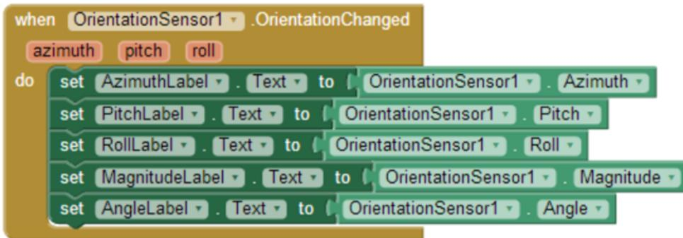
Figure 23-9. Blocks to display the OrientationSensor data
