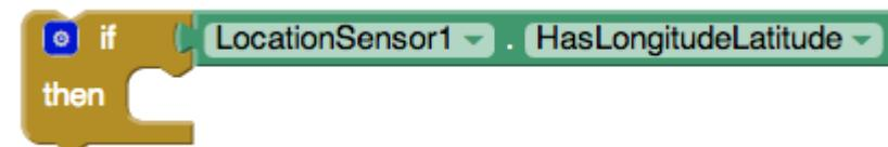
**Figure 23-7.** Testing whether the sensor has a reading by using the `HasLongitudeLatitude` block
