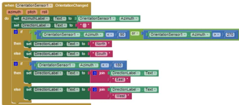
Figure 23-13. Programming a simple compass
