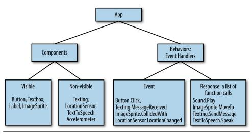
Figure 14-2. The internal architecture of an App Inventor app
