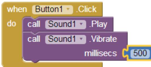
Figure 1-16. Plugging the value 500 into the millisecs socket
