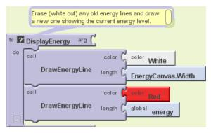
Figure 5-7. Defining the procedure DisplayEnergyLevel
